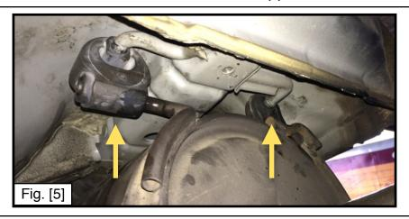
**Step 5.** Raise the EcoHitch into position by lining up the holes in the fame plates with the weld nuts in the frame rails of the vehicle. Secure with (1) M10-1.25x40mm Hex Cap Screw, (1) M10 lock washer, and (1) 3/8" flat washer in each of the weld nuts and hand tighten. Center the hitch on the vehicle and then torque the M10 hardware to 36 ft-lbs. See Figure [6].
